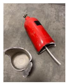
Ruptured fire extinguisher recovered from site.
