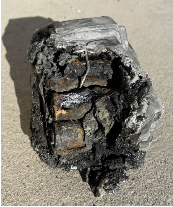
Figure 1 - Damage to battery after being run over
