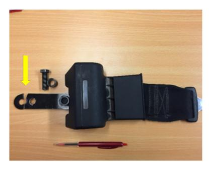
A late model loader was operating at a sand quarry. The operator of the loader drove into the sand stockpile to load his bucket. As he did so the seatbelt bracket failed, and the operator was flung forward striking his head against the cab roof and windscreen. Fortunately, the operator only received a minor neck muscle strain in the incident.
