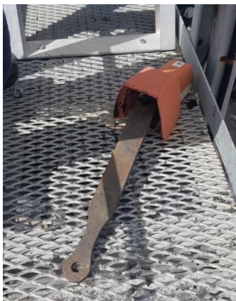
Lever used as weight on deadman switch
