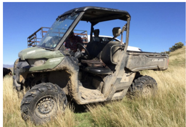
FIGURE 1: The vehicle roll cage was intact and the vehicle was driveable after the incident
