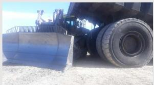
A dump truck reversed into a dozer on a tip head. No injuries were reported and only minor damage was reported. The truck had a broken reversing mirror. The dozer was moving at the time. Mine operators must consider the appropriateness of proximity detection systems to prevent machine interactions.
