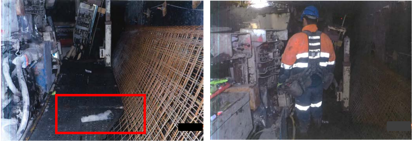
Figure 2 (left) The broken half of the flight bar on the platform of the continuous miner and Figure 3 (right) A simulation of where the injured worker was reportedly positioned when the flight bar hit him
