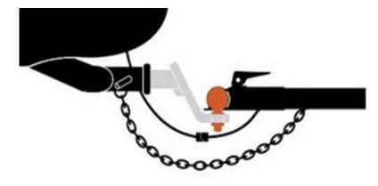
A worker attached a box trailer to a light vehicle in order to deliver a small quantity of rock. The worker attached the safety chain on the trailer to the tow bar bracket on the light vehicle but neglected to put the locking pin into the tow ball fitting.
