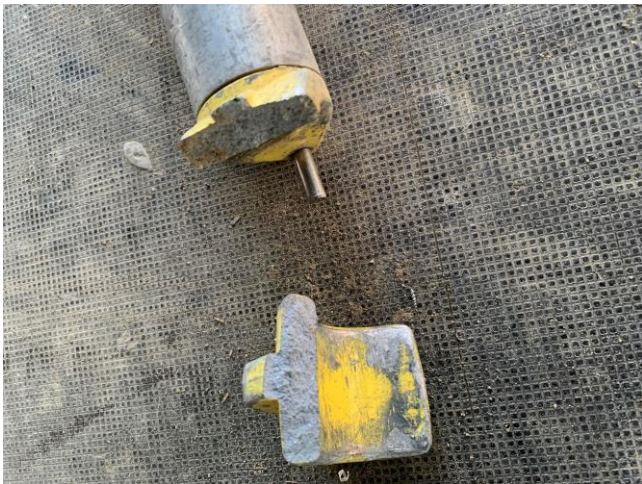
Photo: Broken mobile scaffold quick release claw clamp (grasper)
