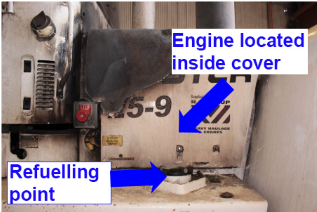
Image 4.2 - Proximity of filling neck to left side of engine cover of OT21.
