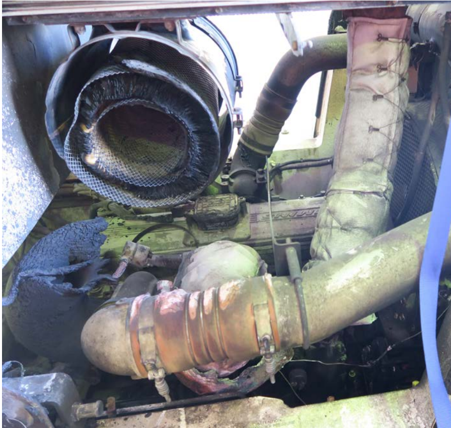
Image 3.13 - Damage inside left-hand engine bay of tyre handler.
