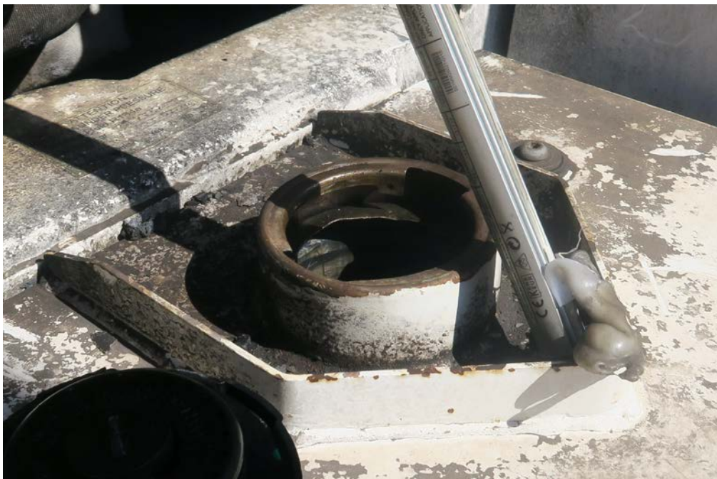
Image 3.5 - Filling neck of Hyster 25-9 tyre handler.
