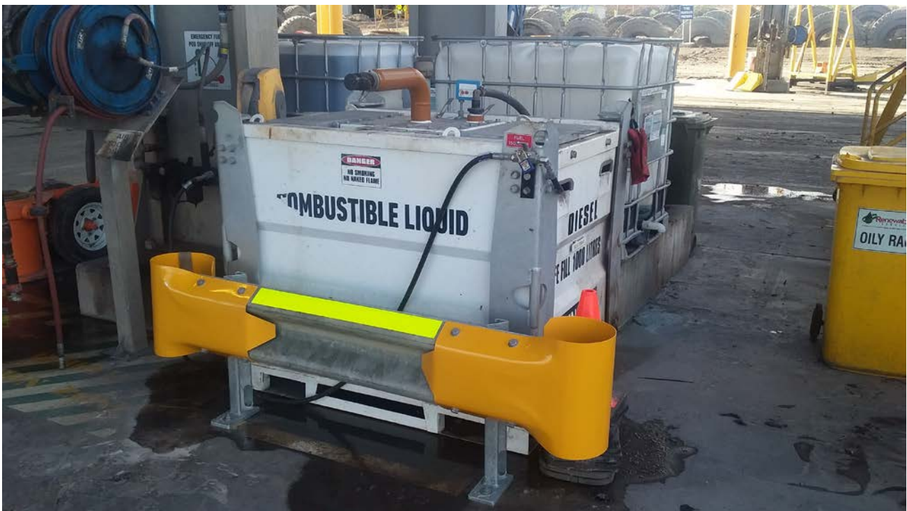
Image 9.1 Low flow refuelling pod installed by the contractor at its tyre bay to refuel tyre handlers.
