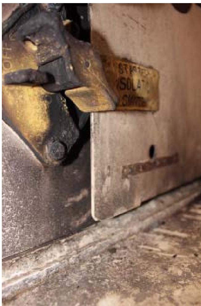
Image 4.1 - Gap between the engine cover and the engine bay frame of OT21.
