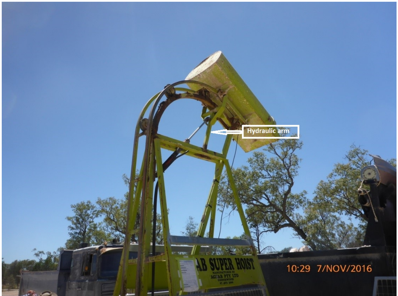
Figure 9: The bucket in tip position (hydraulic arm engaged).
