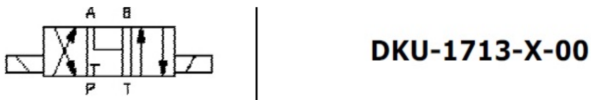
Figure 16: Converted solenoid valve configuration in the system at the time of the incident.
