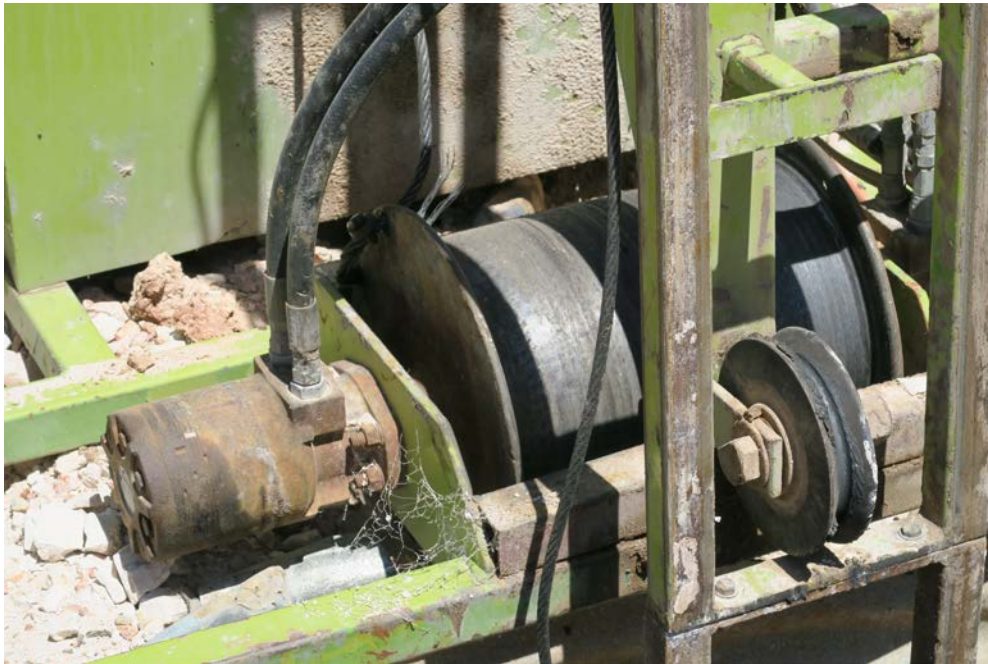
Figure 7: Hoists drum and cable.
