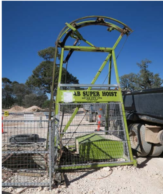
Figure 4: The bucket of the Ag-Fab super hoist.
