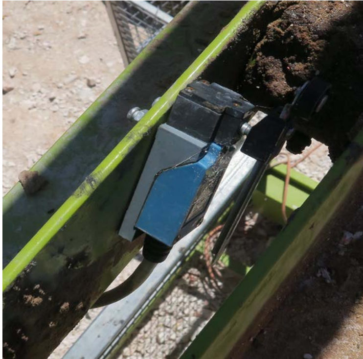
Figure 11: The bucket in the sump (bracket and limit switch).
