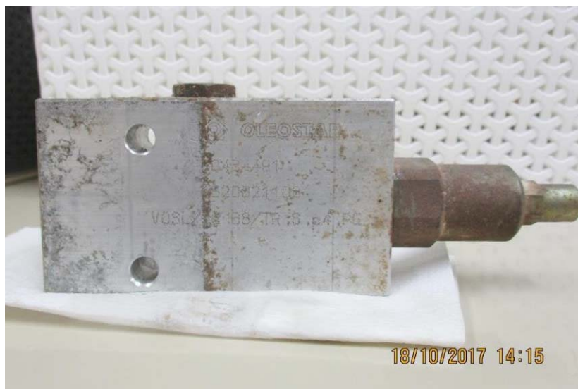
Figure 19: The counter balance valve sized from the hoist.
