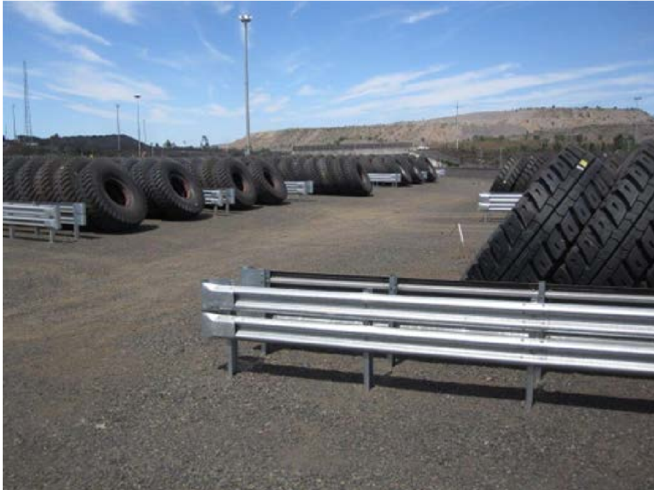
Image 3: Earth mover tyre storage showing segregation and access
