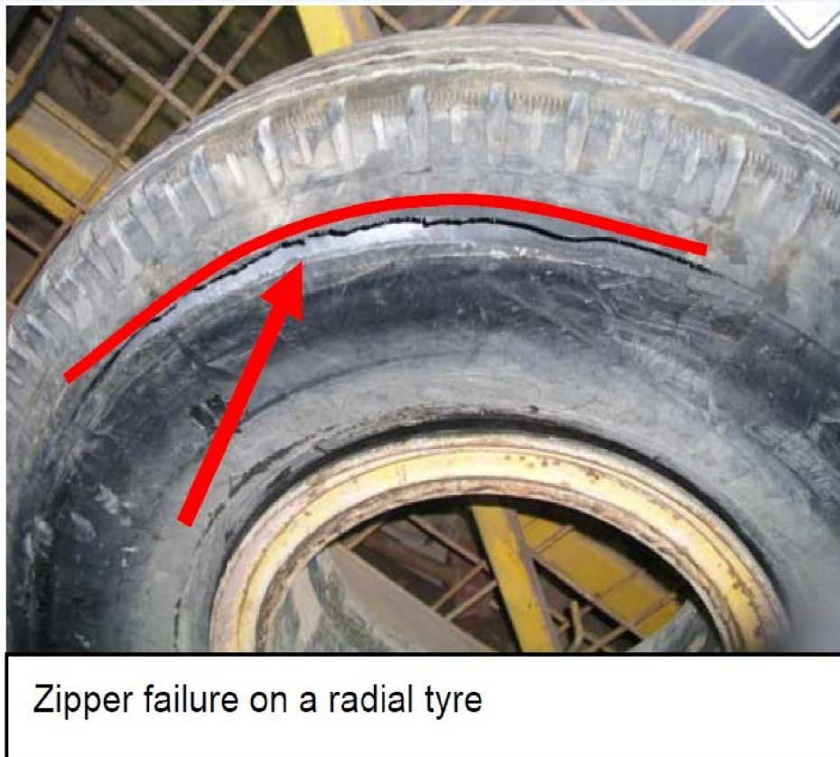
Image 6: Zipper failure on a radial tyre
