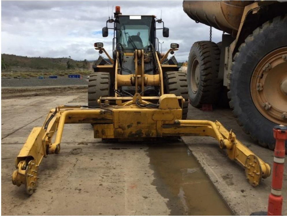
Image 1: A front-end loader with clamp type tyre handler attached
