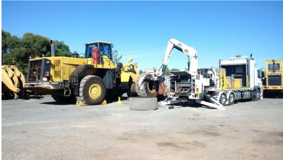
Image 2: Vehicle mounted crane with clamp type handler attachment
