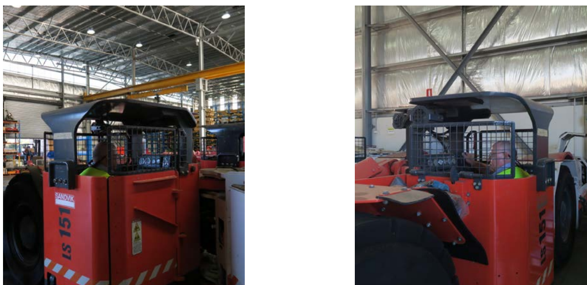
Figure 19: Guarding on a 5 tonne LHD.
