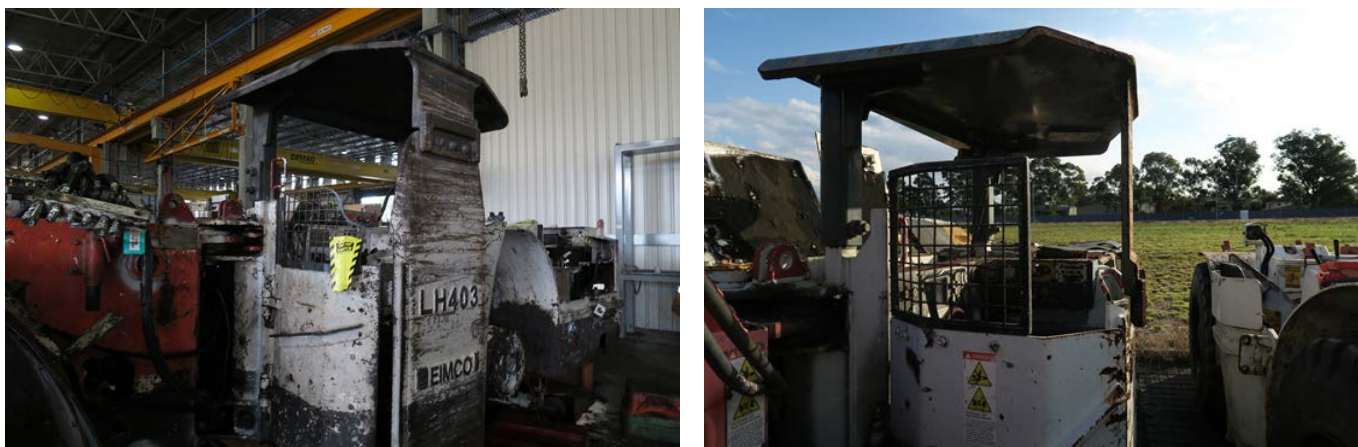
Figure 21: Retrofitted guarding on LHD vehicles.
