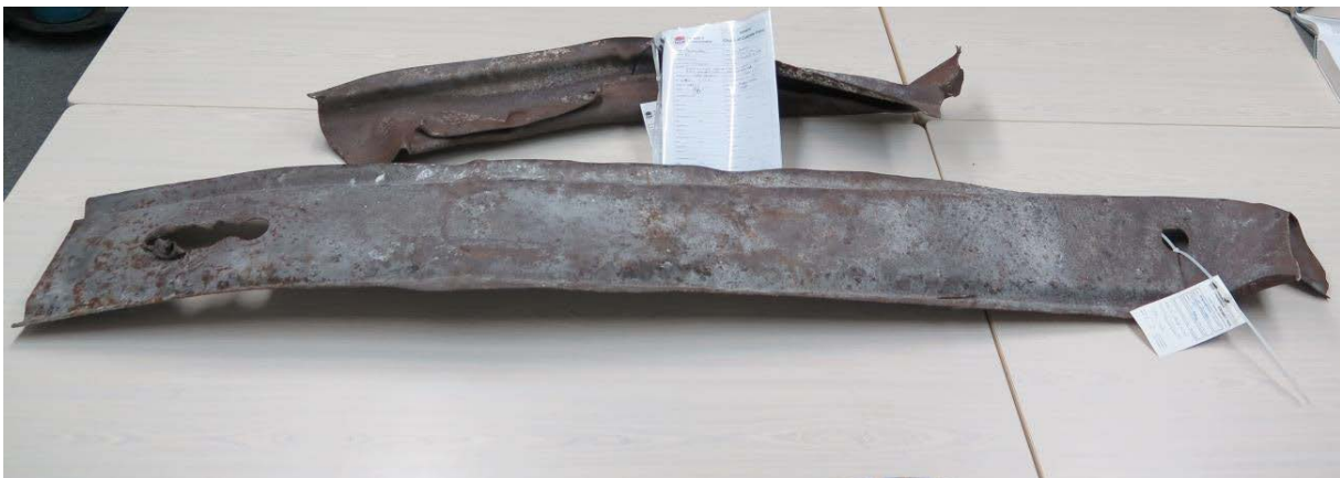
Figure 15: The two sections of damaged W strap.
