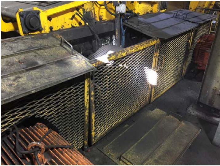
Figure 11: Exposed rotating shafts on conveyor drive.
