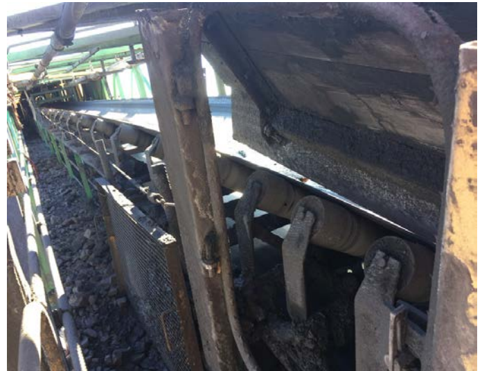
Figure 12: Guard mesh and part of frame corroded.
