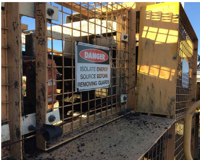
Figures 57 and 58: Lanyard not able to be effectively operated due to proximity to or positioned behind guard mesh.
