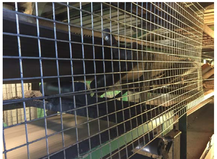
Figures 57 and 58: Lanyard not able to be effectively operated due to proximity to or positioned behind guard mesh.
