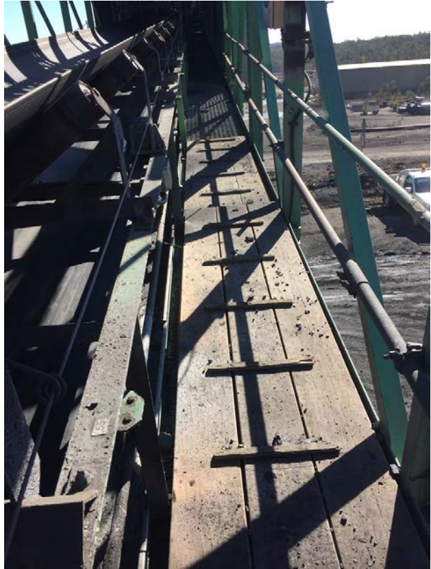
Figures 45 and 46: Rubbish, materials and scaffold boards become trip hazards, especially at the top of stairs
