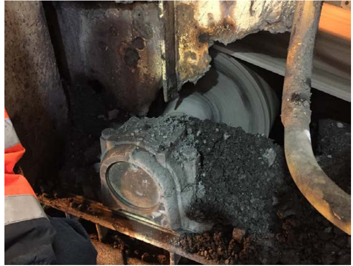
Figure 12: Guard mesh and part of frame corroded.
