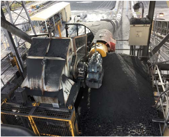
Figure 49: Grease leaking out of bearing seal on walkway.
