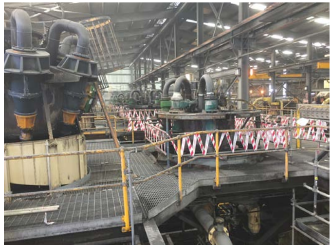
Figure 17: Temporary site fencing restricts cleaning. Figure 18: Tapeused as barrier around low cyclone underpan.
