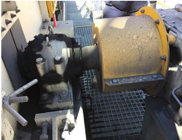
Figure 11: Exposed rotating shafts on conveyor drive.
