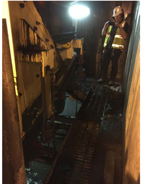
Figures 29 and 30: No protection against falling into cyclone underpan or beside reclaim tunnel vibrating feeder.
