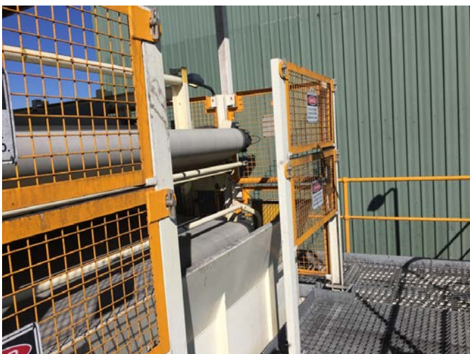
Figure 13: Toggle retainer does not require tool to remove.
