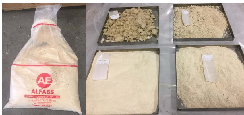
Figure 1: Bat Bag barrier and samples of stone dust obtained for testing.
