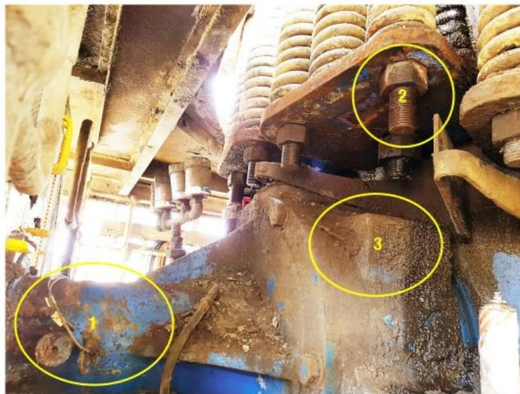
1. Countershaft the fitter was straddling. 2. Nut that was being un-tensioned. 3. Countershaft ledge on which the ram and steel plates was positioned.
