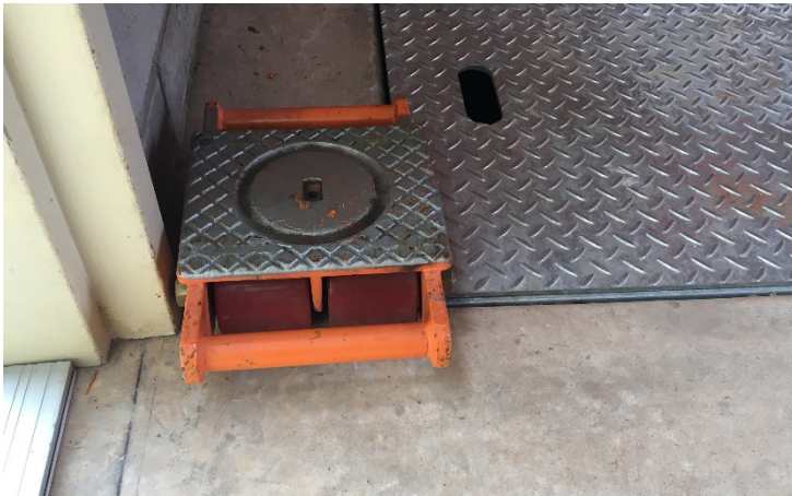
Image 1: The machine skates positioned at the edge of the checker plate most likely contributed to the incident.
