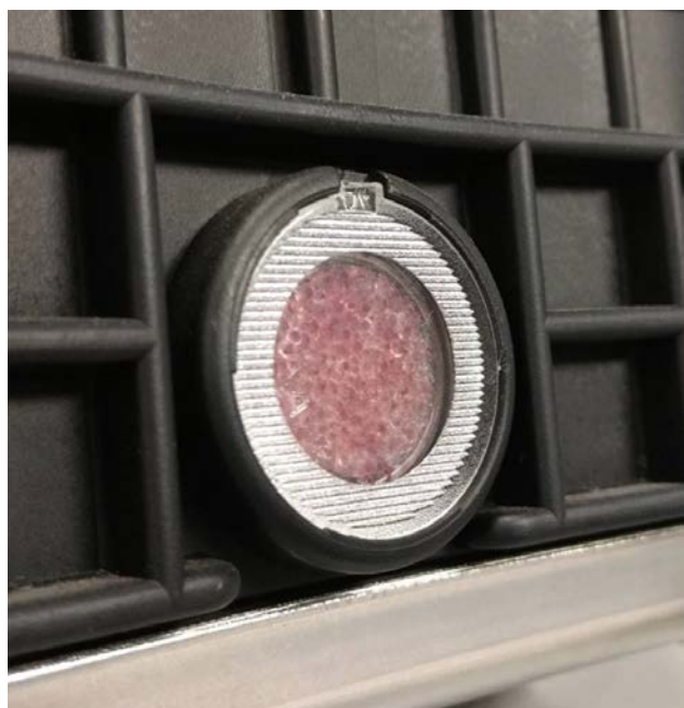
Photo 2: Clean window with moisture indicator visible.
