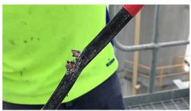
Mine operators must have systems and checks in place for workers to complete pre-use inspections of portable electrical hand tools and monitor worker compliance.
