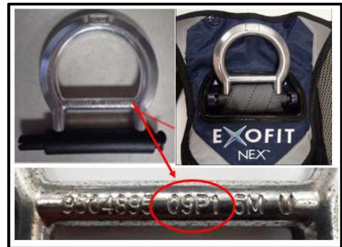
Step 2 Lot Code Stamp Location on D-ring – lot code must be (09P1)
