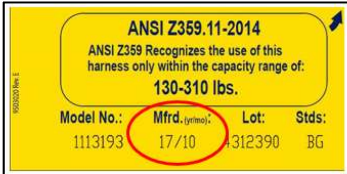
Step 1 Manufacture Date on Harness Shown in Red Circle – must be between 16/01 (2016, January) and 18/12 (2018, December)
