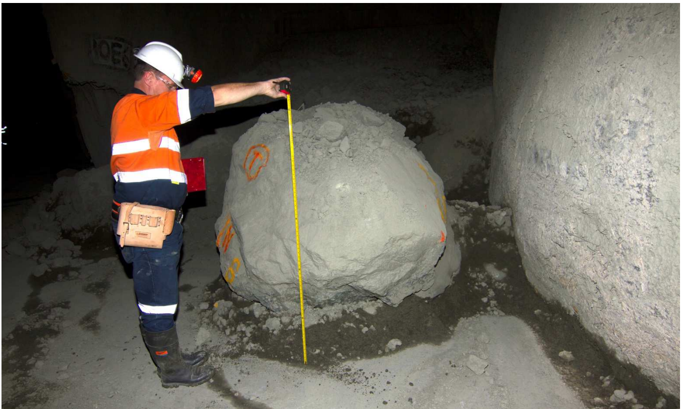
Figure 14 Photograph of a large rock that was contacting the front of the water cannon after excavating around it.
