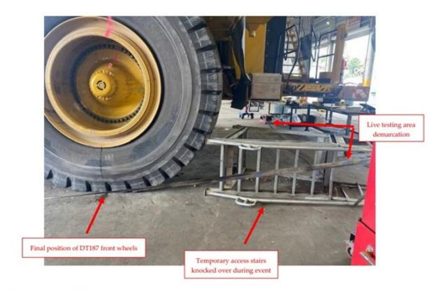
Comments to industry: This incident demonstrates the need for a safe system of work to be in place when conducting function testing. This system should limit workers to a bare minimum required for the testing. Additionally, no-go zones and barriers must be in place and enforced to prevent other workers from entering the work area.
