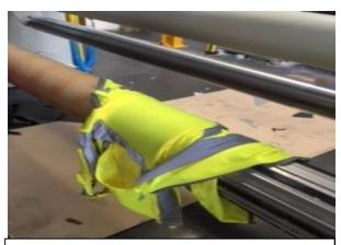
This picture shows the operators vest getting stuck to the adhesive tape on the cardboard former and wrapping around the spindle.
