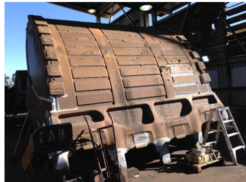
Fig 3. – Alternative wear package with multiple plates
