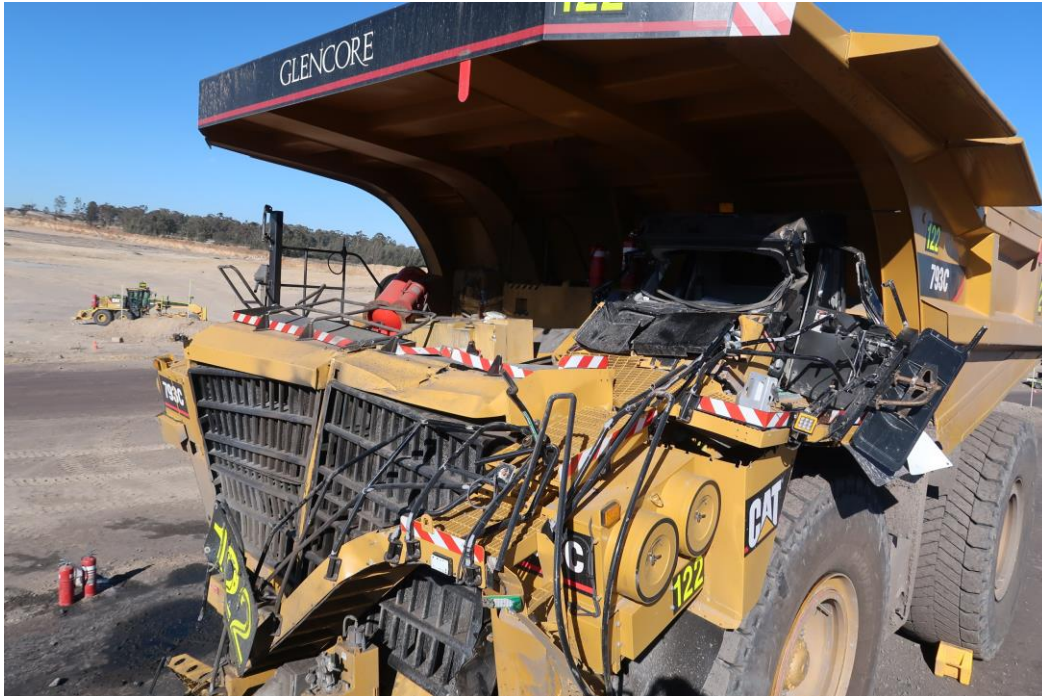
Figure 2: Damage to front and cabin of DT122
