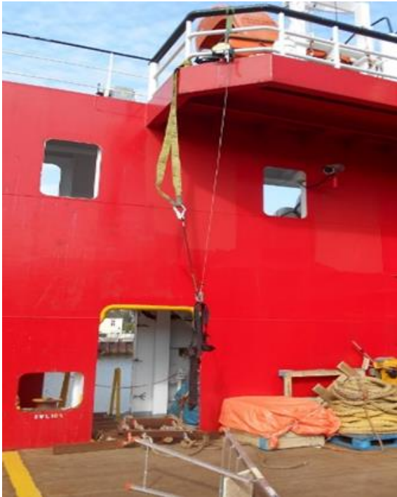
Incident location, with harness hanging from belt, and fall arrestor connected for retrieval, as a demonstration of the situation at the time of the incident. The fallen ladder was part of the drill scenario.
