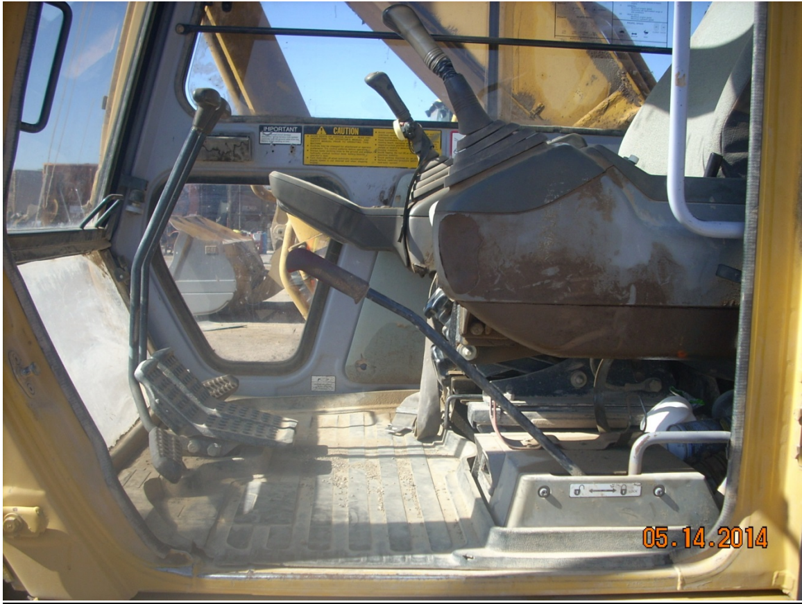
Photo shows the lever in the forward 45 degree position, engaging the excavator's hydraulic system, and making it difficult to exit and enter the operator seat.
