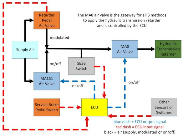
Figure 1: Illustration of the Retarder Control Circuit
