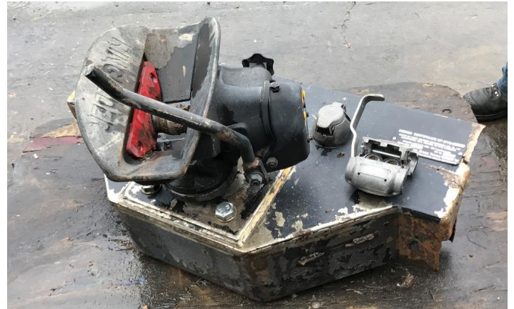
After several months in service, cracks developed where the main body of the drawbeam attached to its side plates, resulting in the trailer's detachment from the towing vehicle.
