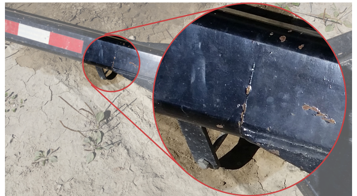
Crack identified on trailer's drawbar after approximately 2 years in service.
