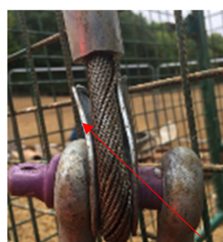
Damage sustained to chassis and steel winch wire thimble
