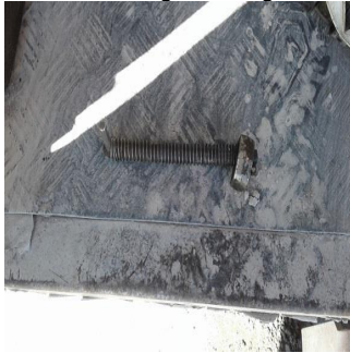
Bar used to by-pass system
