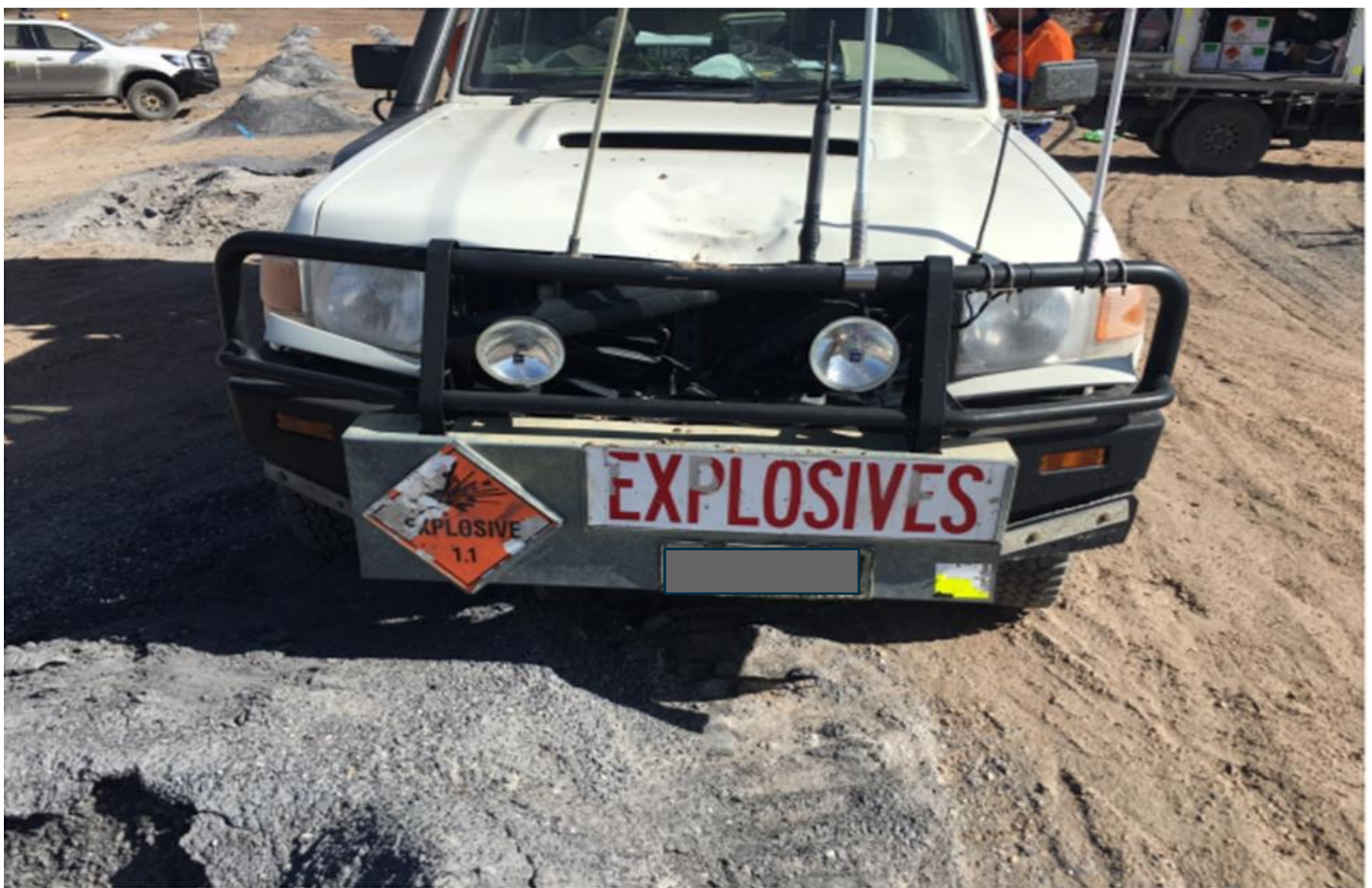
Photograph 1: Damage to bonnet and front grill of light vehicle caused by flyrock.
