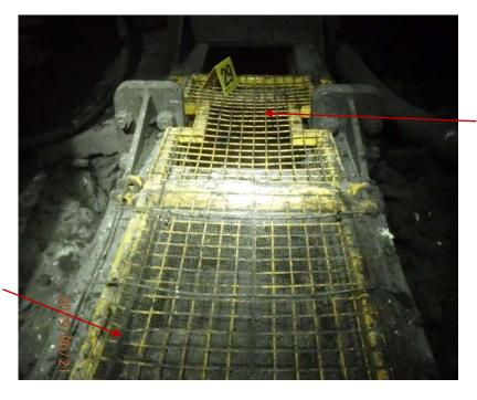
Reinforcement mesh overlayed by tech mesh on top of a fixed guard. Foot entered conveyor and was trapped.
