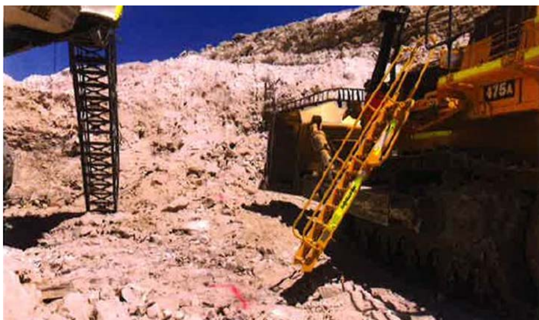
Figure 3 – Excavator reverses into dozer (SInNot-2018/00355). Photo courtesy of the mine.
