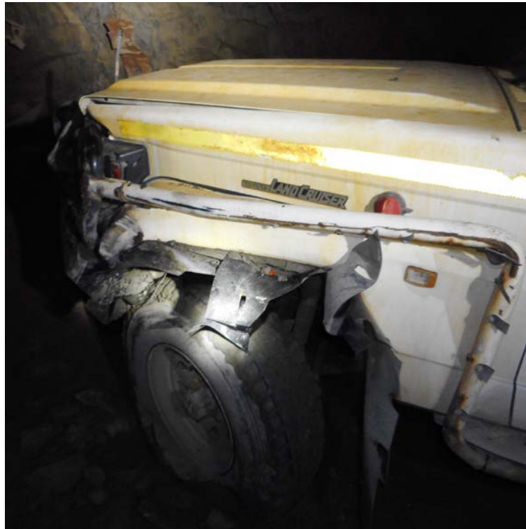
Figure 4: Haul truck hits light vehicle (IncNot0033912). Photo by NSW Resources Regulator
