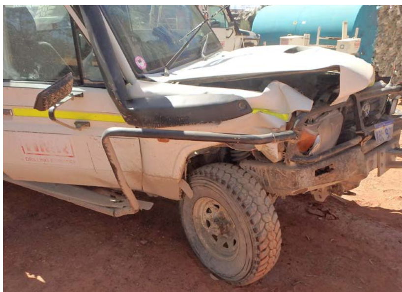
Figure 2: Heavy contact with decline wall (IncNot0033889). Photo by NSW Resources Regulator
