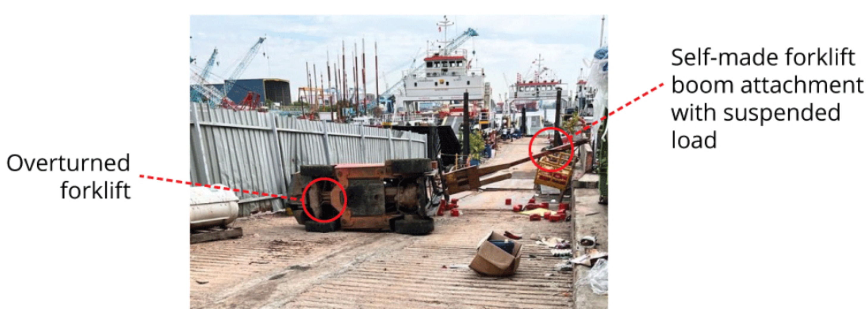
Overview of accident scene.
