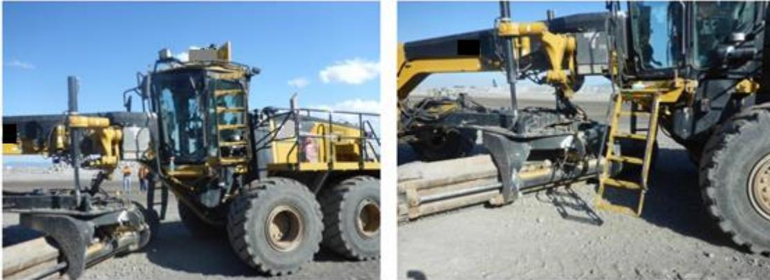
**Figure 7 - Raised and lowered positions of grader access ladder**
