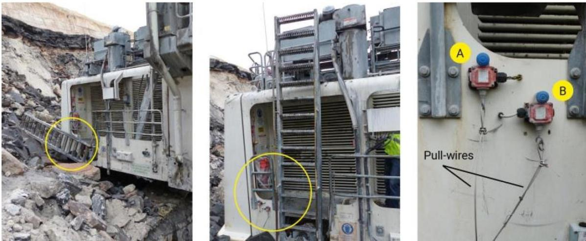
**Figure 6 - Scene of fatality caused by shovel hydraulic access ladder**
