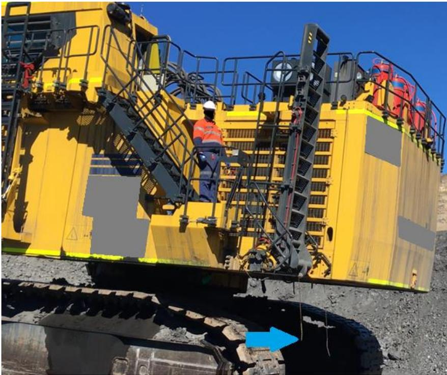
**Figure 5 - Pull-chain for the ladder emergency release valve**
