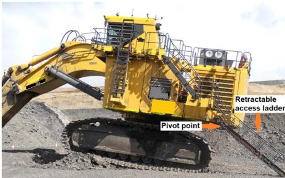
Figure 1 - Excavator with retractable ladder
