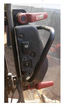
Figure 2 - D-Series secondary exit handles
