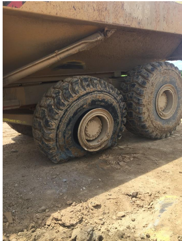
Photo 2 - Deflated position 3 tyre
