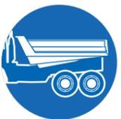
Dumpers **stored energy** is held in both the vehicle itself and in the load it is carrying. Lowering the dumper tipper, when not actively required, removes the stored energy from both of these elements.
