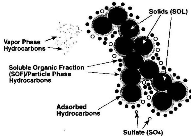
**Schematic – mine diesel particulate
