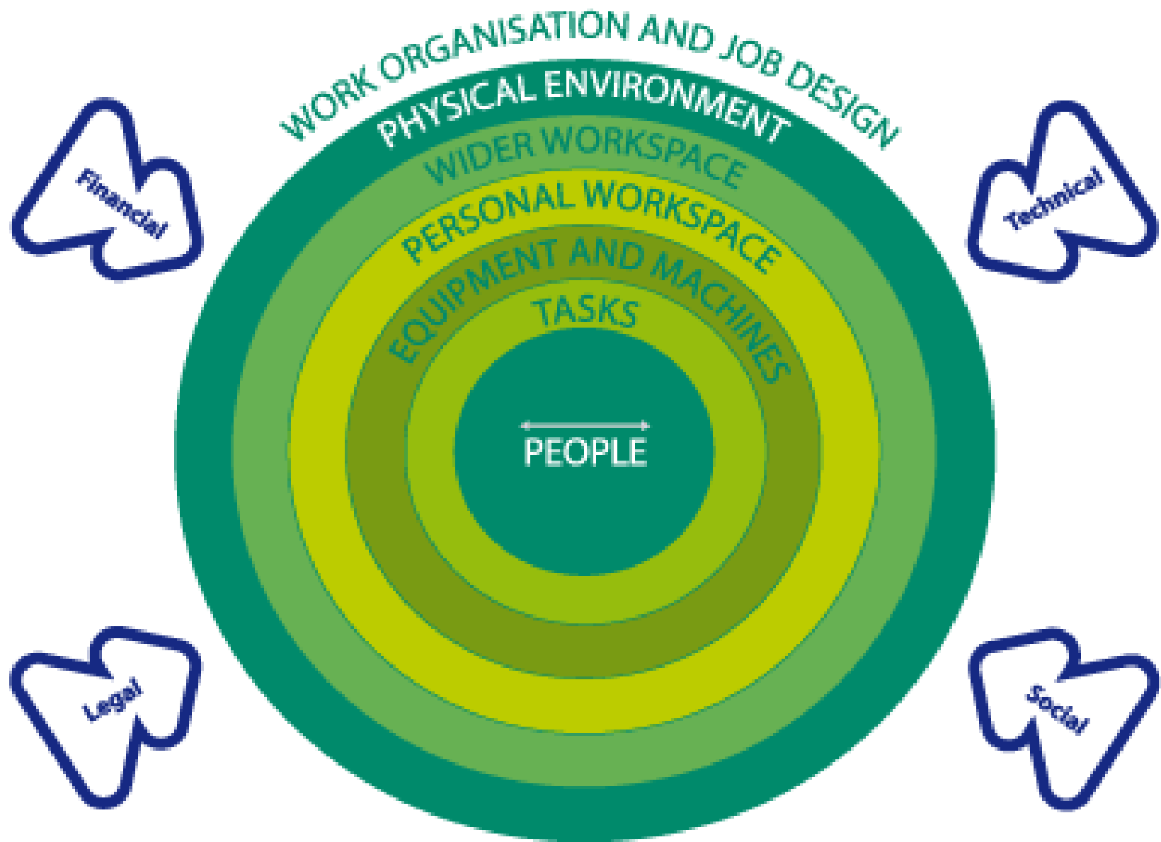
'Concentric Rings' - Model of ergonomics factors relevant to work design. (Adapted from Grey et al., 1987, as in Wilson and Corlett, 1995)
