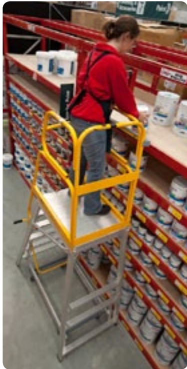
Figure 18: To access stock a worker uses a step platform with barriers on all sides.
