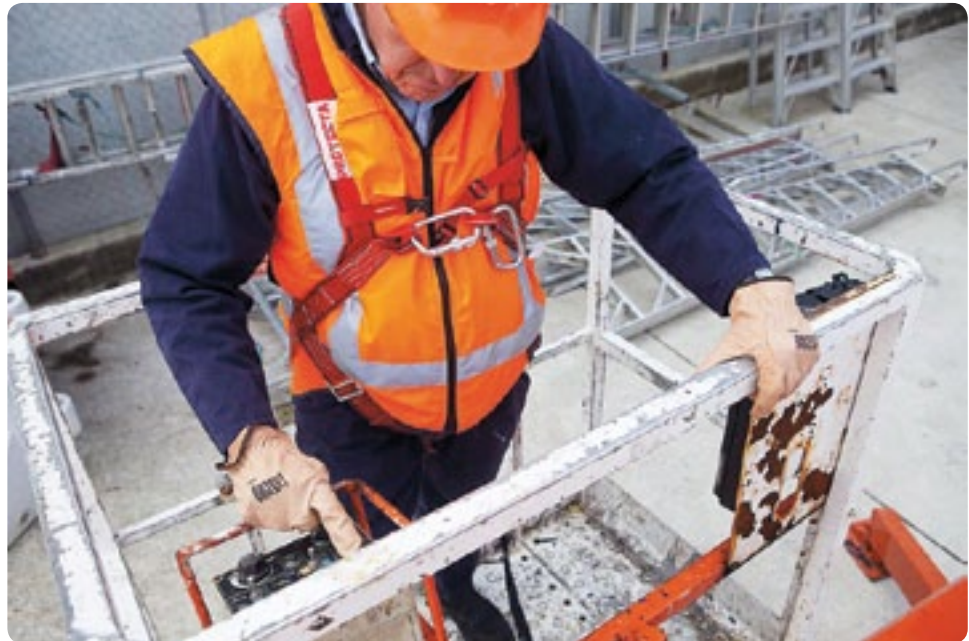
Figure 9: A worker restrained in a boom-style elevating work platform.
