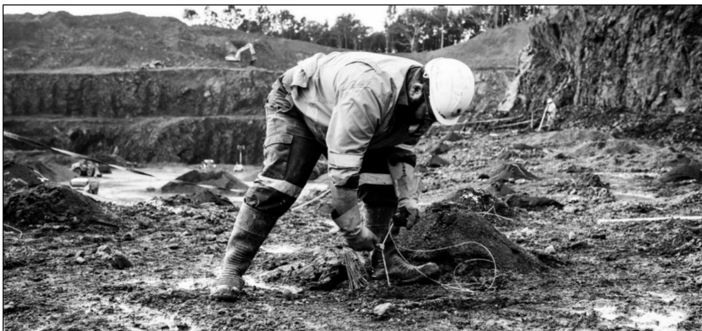
The sequencing of blastholes permits the controlled release of explosive energy in a manner that provides the required level of confinement and burden relief to achieve the desired fragmentation and blast movement, while minimising the risk of undesired outcomes such as flyrock, overpressure, vibration, noise, misfires and poor fragmentation.
