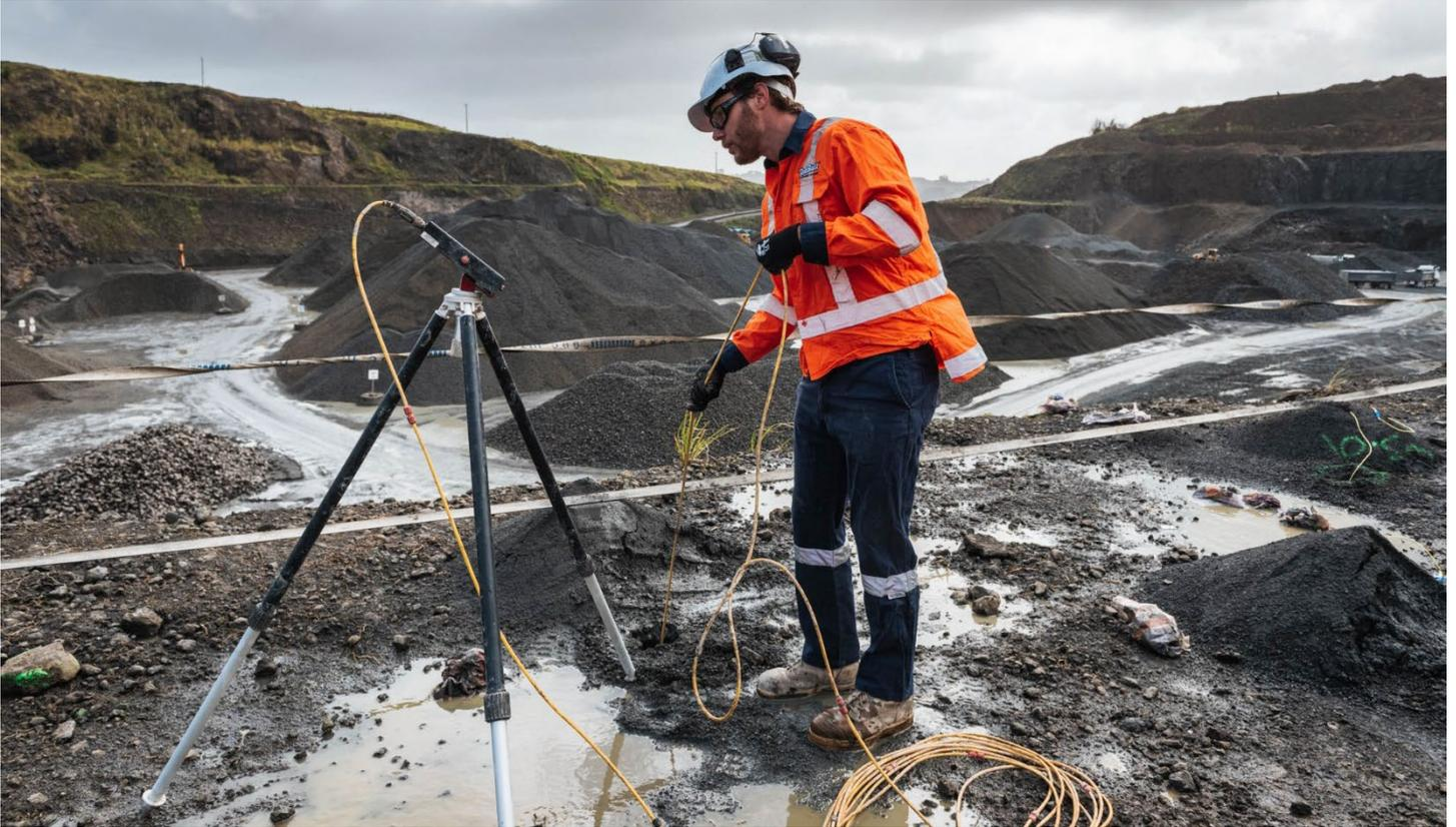
All blastholes must be measured prior to charging, in the event that re-drills or adjusted charging is required. If measurement was carried out prior to the day of charging, and a physical change to the blasthole is likely (e.g., following a rain event), then it is recommended that blastholes be re-measured prior to charging.
