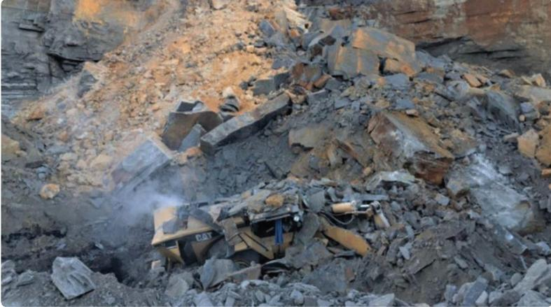
When mine/quarry faces are exposed, relaxation of the rock occurs which may lead to loose material falling or rolling from the face.
