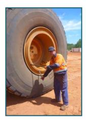
a single fitter manually used two levers (pictured) to remove the ring that on average weighs 43 kg. In addition to the musculoskeletal injury risks, there were also significant safety risks of a
