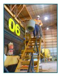
to clean out the air filter. The person then carries the filter back up the stairs and repeats the process again. The filter needs to be cleaned on the ground because of the excess dust produced when using the standard air wand. Not only is there significant musculoskeletal injury risk, bust there is also significant risk of falling down the stairs.
