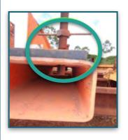
into the jib, personnel simply use a rattle gun to screw the bolts down against the fork tines creating the desired angle that matches the front strut assembly. This improvement has eliminated the potential of hand crush injuries and line of fire injuries as no more packing is required.
