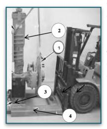
compensate for the strut assembly angle. Despite the adjustment this still posed risks of hand crush injuries and line of fire issues if the packing was to dislodge due to unplanned movements as the assembly weighs
