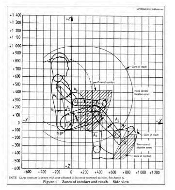
Figure 2: ISO6682: Earth-moving machinery - Zones of comfort and reach for controls.
