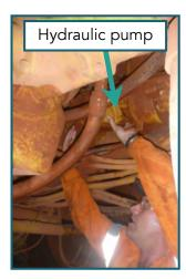
the pump, which required excessive upper limb exertion. To make this job even more difficult personnel often had to manoeuvre various hydraulic hoses with one hand, and use the other hand to access the pump. A high risk of pinch points injuries was also
