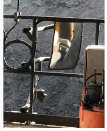
1.12 Truck handrail impedes vision for smaller truck drivers
