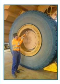
high (dependent on wheel rotation), some operators would have to strain to reach up high. Other operators even reported climbing within the rim to take tyre pressures. Significant safety risk was also related to the possibility of tyre failure due to the enormous Pinch Point
