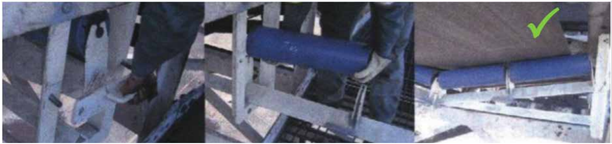
Figure 13: A slide for return rollers which forgoes heavy manual lifting
