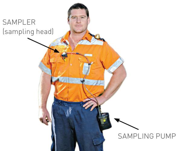
Figure 4: Personal dust sampler
