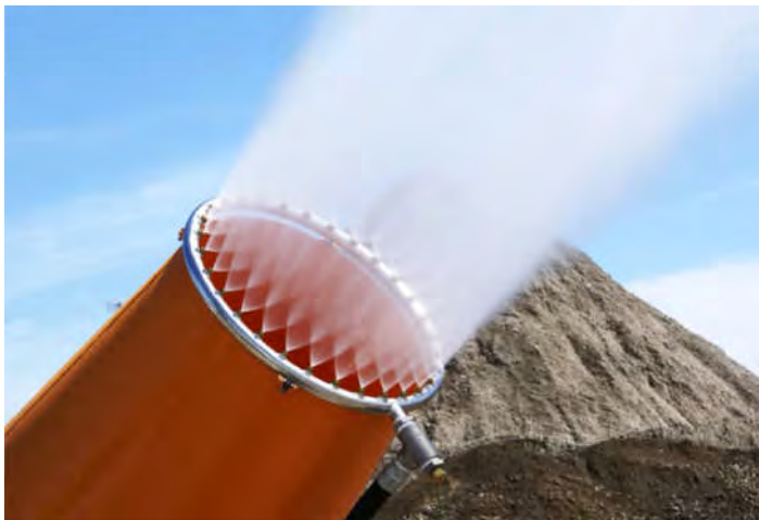
The DB-60 Fusion forces water through a circular stainless steel manifold with 30 atomising spray nozzles
