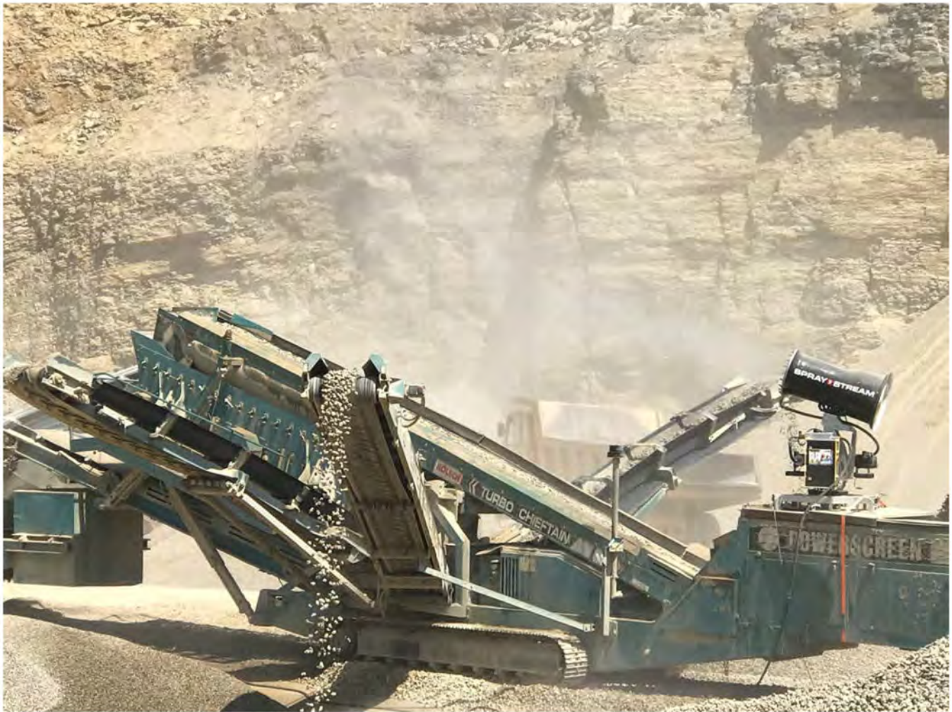
A Spraystream system fitted to a three-way split screener in operation at a quarry in Germany
