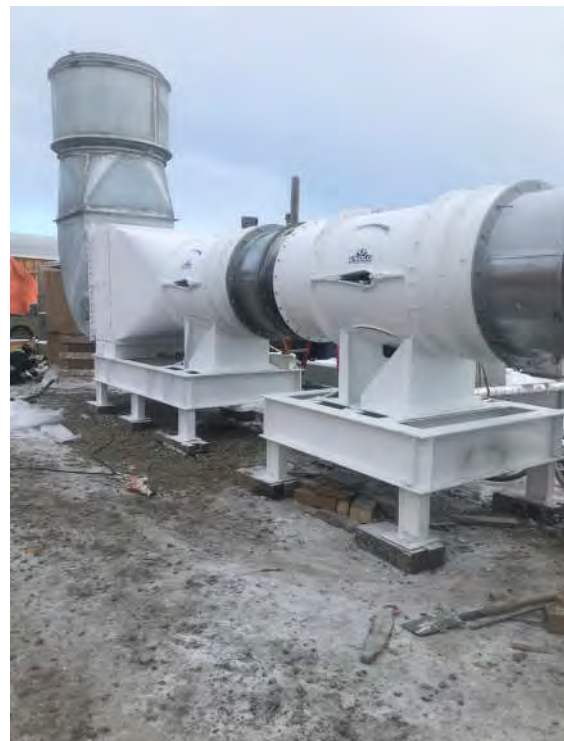
A wet dust extractor unit at work on a tunnel
