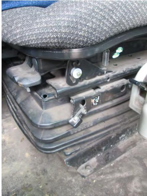
1.8 Seat height cannot be adjusted to suit leg length of small operators
