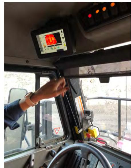
7. Retrofitted cab equipment: smaller operators reported excessive reach required to operate the dispatch screen and radios.
