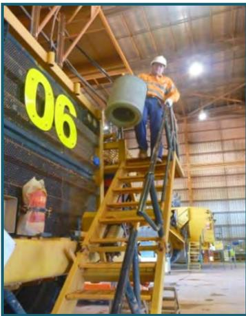
The person then carries the filter back up the stairs and repeats the process again. The filter needs to be cleaned on the ground because of the excess dust produced when using the standard air wand. Not only is there significant musculoskeletal injury risk, but there is also significant risk of falling down the stairs.
