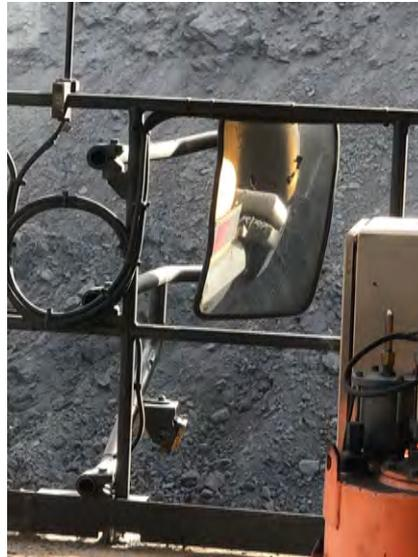
1.12 Truck handrail impedes vision for smaller truck drivers
