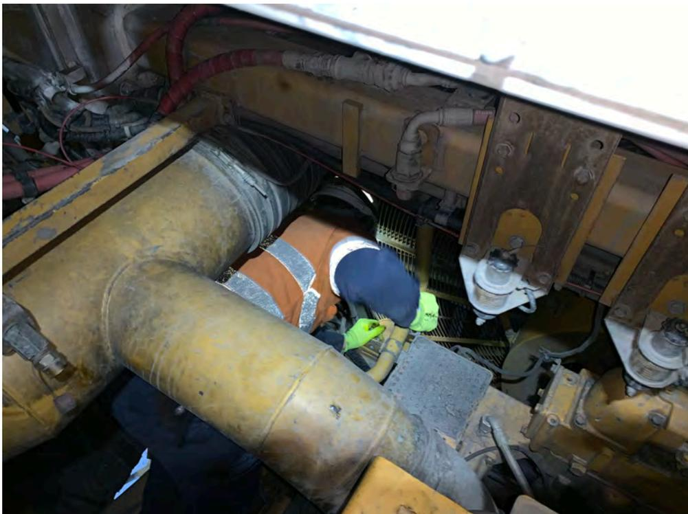
22. Removing and replacing dozer “belly guard”: weight is approximately 300kg but up to 700kg when loaded with stones and dirt. A jack (TED) has been designed to assist with task. The maintainers suggested a control where a tractor fitted with a hydraulic arm and remote control could walk it out. CAT provide a tool but maintainers indicated it was not adequate. Maintainers reported potential for crush injuries to arms/hands/legs and fatalities associated with this task.
