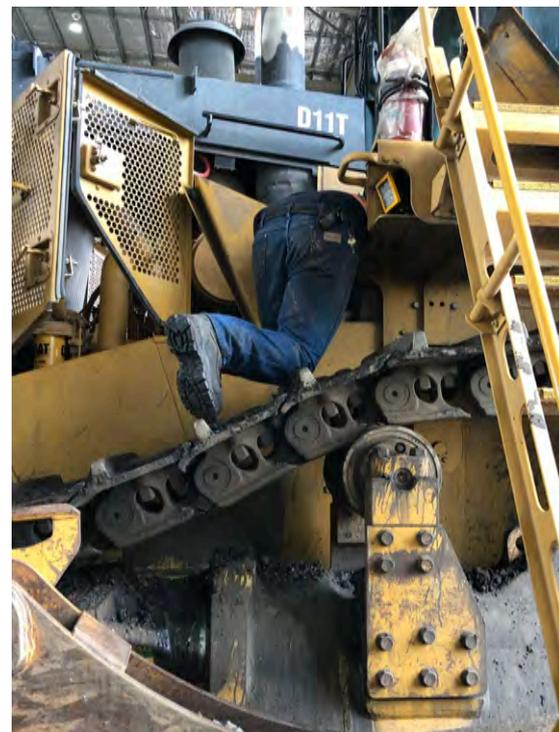
24. A number of sites had fabricated plates to make access easier for dozer maintenance, either to fit between tracks, or on front of the dozer.
