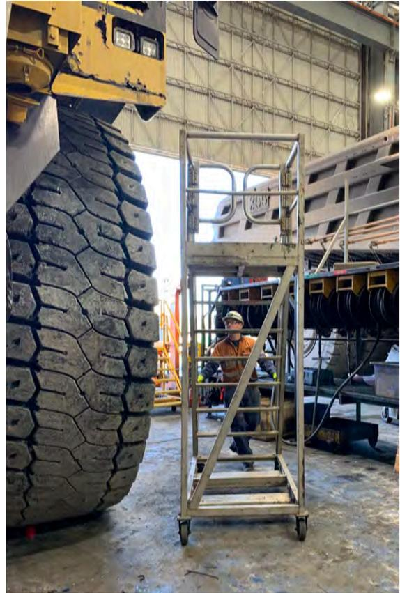
19. Changing haul truck air filters: maintainers are required to adopt awkward postures to access the filters. The internal pressure makes taking old filters out difficult, and they are heavy and dirty. The task is undertaken by standing on the stair plate and leaning out. Different solutions have been developed at different sites.
