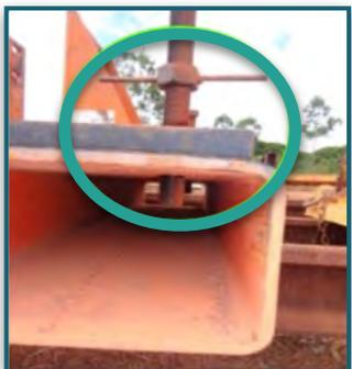
into the jib, personnel simply use a rattle gun to screw the bolts down against the fork tines creating the desired angle that matches the front strut assembly. This improvement has eliminated the potential of hand crush injuries and line of fire injuries as no more packing is required.
