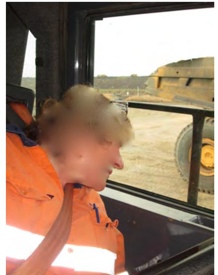
9. Dozer seats were considered particularly problematic as they require the operator to sit awkwardly during operation. Suggestions were made to have the seat and console move as one unit as is the arrangement in scrapers. Dozer operators estimated more than 50% of their shift was spent with their body/neck rotated to enable them to look over their shoulder to see where they were operating.
